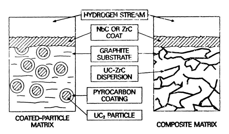
Comparison of the fuel structure in the standard, coated-particle, graphite matrix with the composite matrix fuel. The continuous, webbed UC-ZrC dispersion prevents hydrogen, entering through cracks in the top coating, from eating deeply into the graphite matrix.
